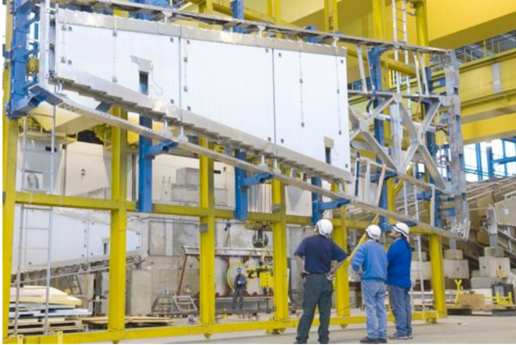
Figure 3.20: A picture of an assembled ATLAS Muon Spectrometer End-cap Sector, along with support structures [1].
