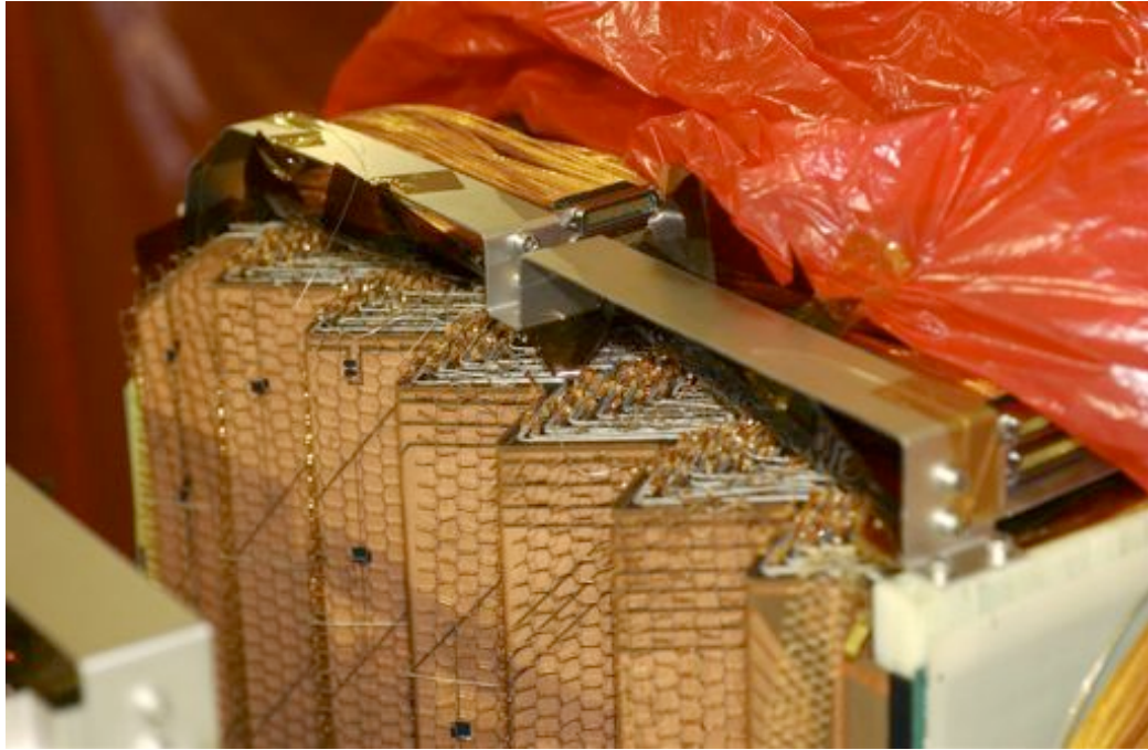
Figure 3.14: A picture of the accordion structure used in the ATLAS electromagnetic calorimeter [1].
