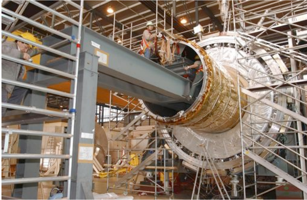
Figure 3.23: A picture of a test insertion of the ATLAS solenoid into the ATLAS EM Calorimeter [1].
